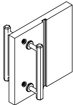
3. On the other side, feed through backplate 1 through the protruding long screw.
